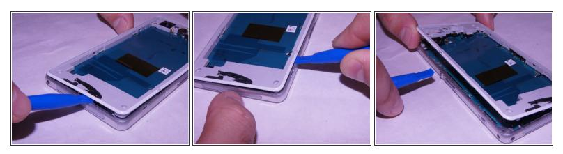
Wedge the plastic opening tool under the back frame. Move the plastic opening tool around the entire frame to separate it from the adhesive.
