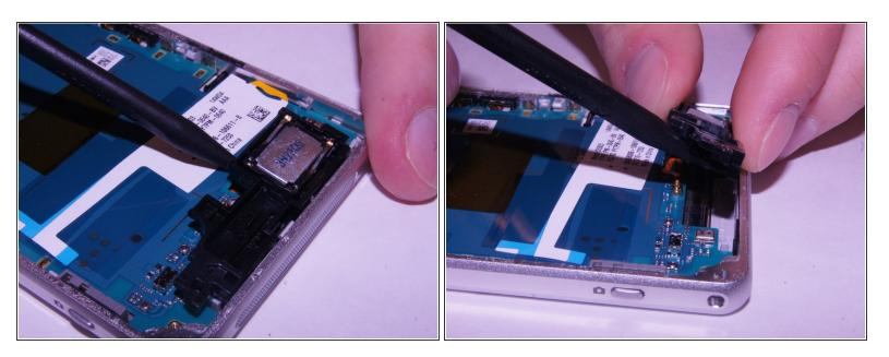
Wedge the spudger underneath the external speaker. Pull up on the external speaker using the spudger.
