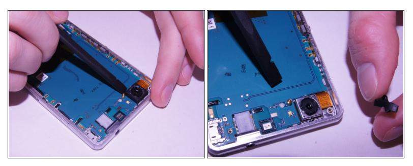
Remove the square rubber gasket from the camera using the plastic spudger.
