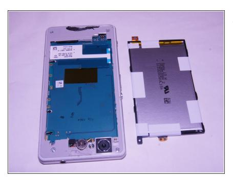
Remove the battery from the device
