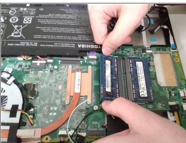
Push outward on the clamps holding the RAM in place.
