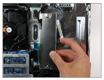
Pull the inverter away from the chassis and lift it slightly out of the rear case.
