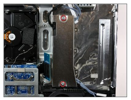
Remove the two 13 mm T10 Torx screws securing the inverter to the rear case.
