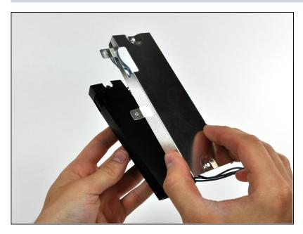
Lift the metal case off the inverter.
