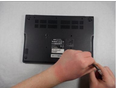
Remove the thirteen 6.0mm screws on the back panel using your Phillips #1 screwdriver.
