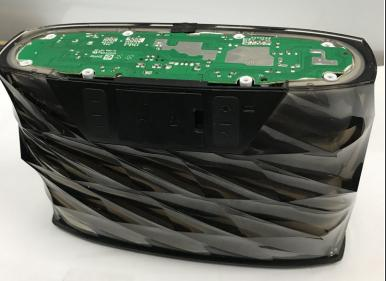
Once the screws are all out, the cover should come off revealing the motherboard.
