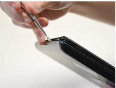
Continue to separate all of the clips around the device until the back cover comes off completely.
