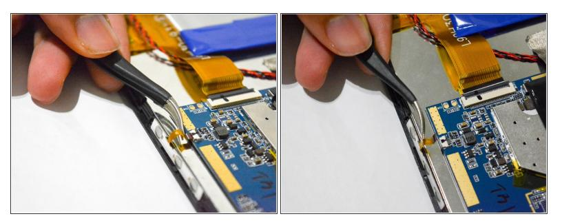
Once the tab is released, use the angled tweezers to take out the tab.
