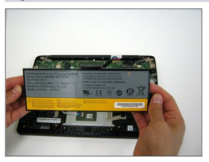
• Lift the battery from the frame.
