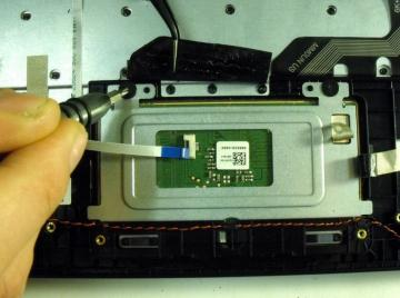
Use a Phillips #00 screwdriver to remove the two 2 mm screws securing the metal plate that holds the touchpad in place
