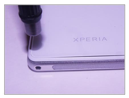
Heat along the edges of the back cover using a heat gun to soften the glue.
