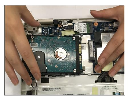
After pulling up on the hard drive, pull in the opposite of the direction of the white barcode.
