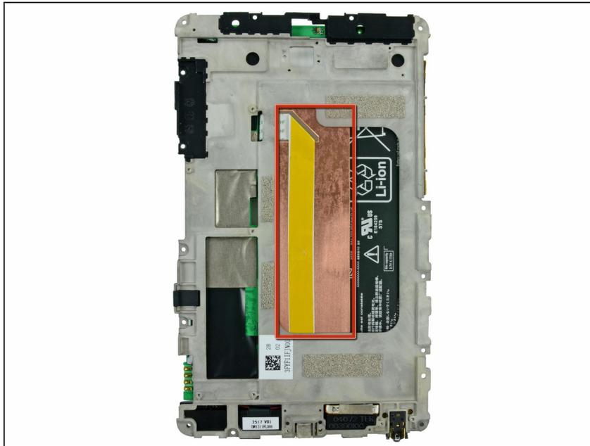
**i** The display assembly is held in place by a large amount of adhesive on the underside of the large copper ESD shield. In the next few steps, you will be using a plastic spudger to release this adhesive.
