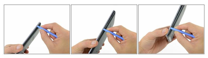
Insert the plastic opening tool between the rear panel and the front panel assembly near the power button and pry up at several points along the right edge of the Nexus 7.
