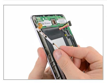
Remove the power and volume button ribbon cable from the Nexus 7.
