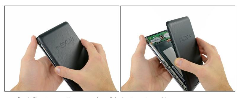
Gently lift and remove the rear panel up off the front panel assembly.
