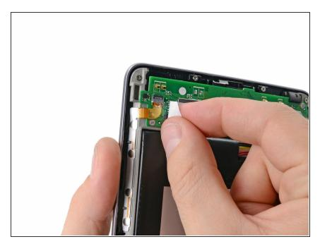
Peel back the label covering the power and volume button ZIF connector.
