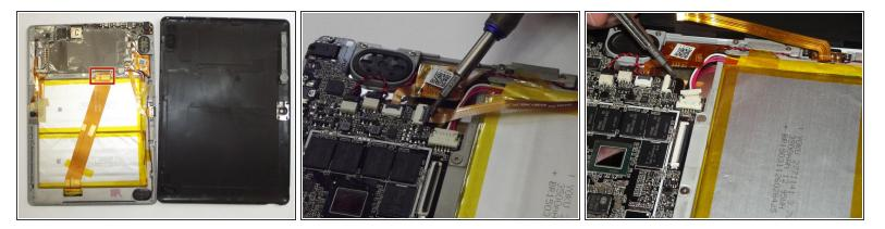
• Remove the smaller ribbon clip on the right side of the device and top right of the battery.
