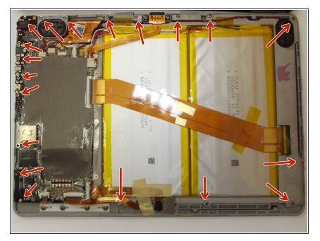
Once you have the cover off, remove the screws from the outer perimeter of the board assembly with a small philips head screwdriver. See arrows.
