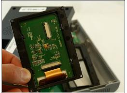
Disconnect the ZIF connector, by using the plastic opening tool to lift up on the small locking flap.
