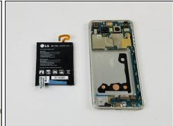
• Firmly pull the blue tab. Be careful not to bend the battery as you pull it away from the adhesive.
