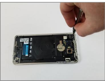
Using a Philips 000 bit, remove 11 screws from the highlighted locations.
