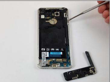
With the screws removed, remove the lower frame components, followed by the upper mid-frame. Both components can be removed with a little prying.
