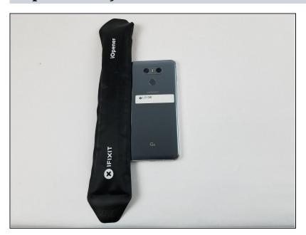
Apply the heated iOpener to the edge of the phone for about 2 minutes.
