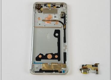
• Gently pry the USB-c port assembly out of the frame.
