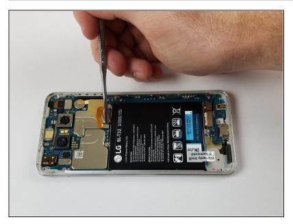
Begin battery removal by very gently prying off the power ribbon with a plastic card or a nylon spudger.
