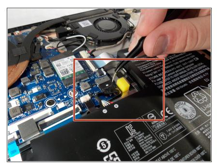
Disconnect the battery by pulling its cable away from the hinge with a pair of tweezers or your fingers.
