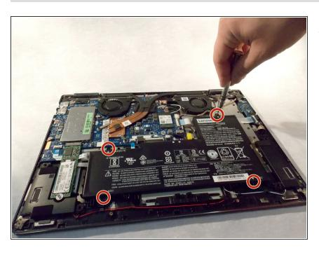
Remove the four 3.5 mm screws around the battery using a Phillips #1 screwdriver.
