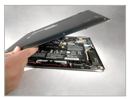
Lift and remove the back cover.
