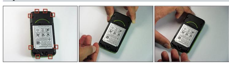
• There are eight snap hooks located around the outer case. Carefully snap these to remove the outer case.
