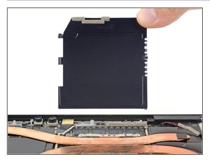
• Remove the heat sink shield.
