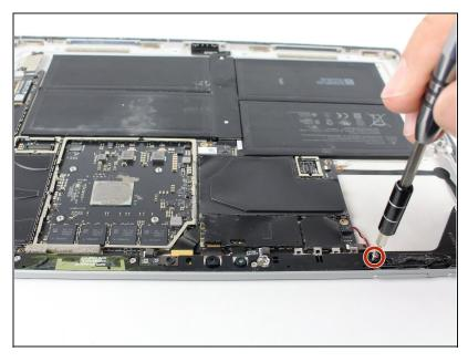
Remove the Torx T5 x 6mm screw connecting the black tie bar to the power button/volume control/speaker assembly.
