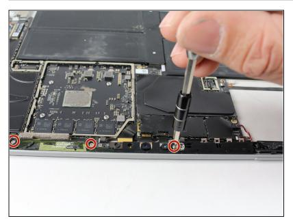
Remove the remaining three Torx T5 x 4.5mm screws holding down the camera tie bar.
