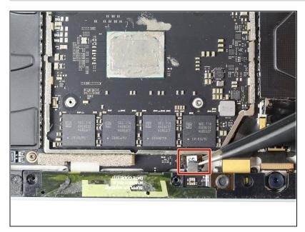
Disconnect the small ribbon cable connecting the camera tie bar to the motherboard by pulling up with tweezers.
