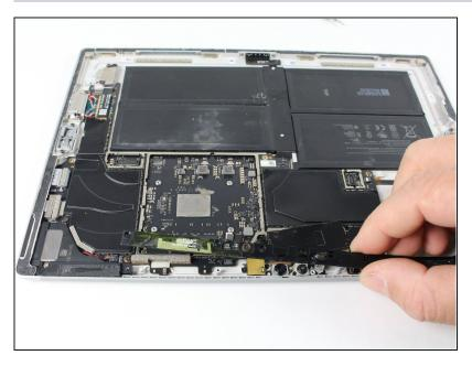
• Lift the camera tie bar off of the device.
