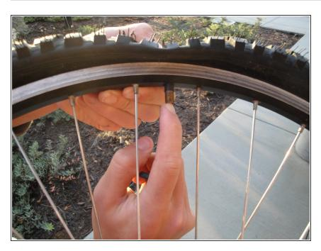
Press the valve core while applying pressure to the tire to deflate the tire.
