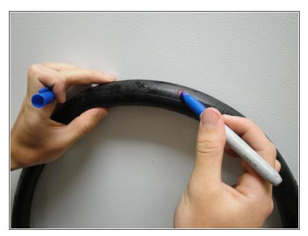
Mark the hole with a marker, and completely deflate the tire.
