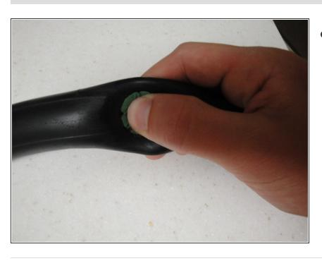
Apply pressure to the patch until the rubber cement is dry.
