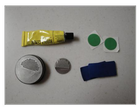
Select a patch kit that you will use to patch the hole. Try to pick a patch that is appropriate for the size of the hole.
