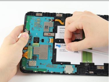
Remove the adhesive film, lift the retaining tab and withdraw the white speaker ribbon.
