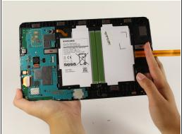
Lift the retaining tab and withdraw the black LCD ribbon.
