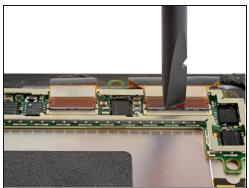
Use a spudger to flip up the small locking flaps on the display cable ZIF connectors.
