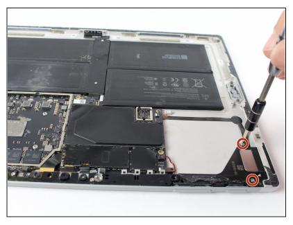
Use a Torx T5 to remove the two 4.5mm silver screws on the power button/volume control/speaker assembly.
