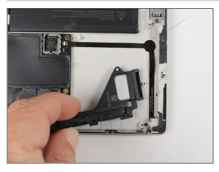
Pull the assembly to the left with hands and lift up to remove.
