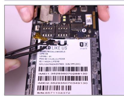
Slowly lift the vibration motor away from the frame and peel up the tape.
