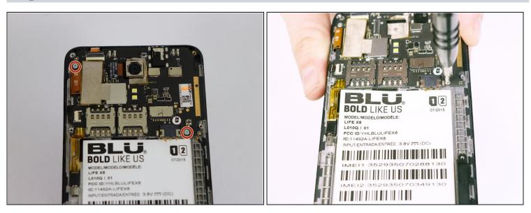
• Use the Phillips #00 Phillips bit to undo the two 1.5mm screws from the motherboard.
