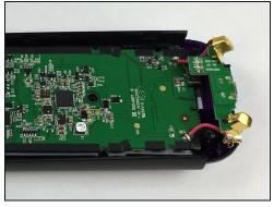
• Use the J0 Philips Head Screwdriver to remove the 5 6mm screws.
