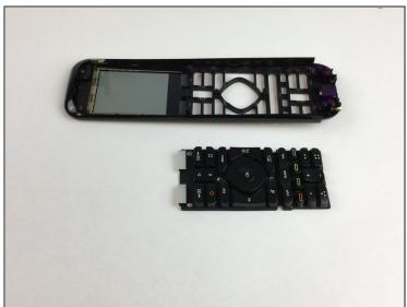
• Use the Blunt Tweezers to carefully remove the keypad from the cover of the remote.
