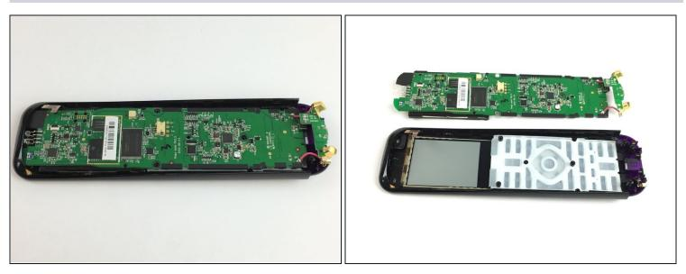
• Pull the circuit board off of the case. Start from the bottom, and lift up to completely detach it from the cover.
