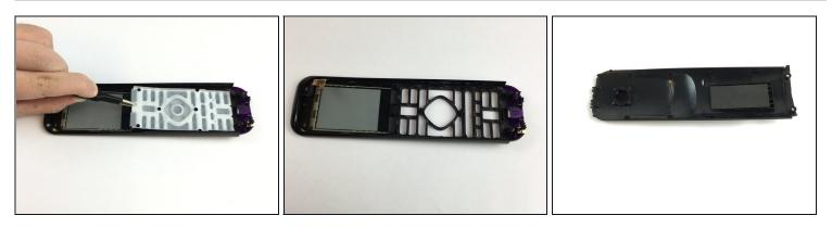
• Use the Blunt Tweezers to carefully remove the keypad from the cover of the remote.
