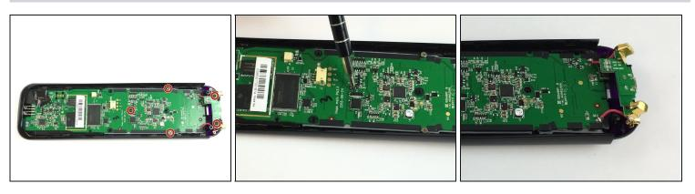
• Use the Phillips #0 screwdriver to remove the (5) five 6mm screws. Keep in mind that once the screws are off, the circuit board will be completely separate from the case.
