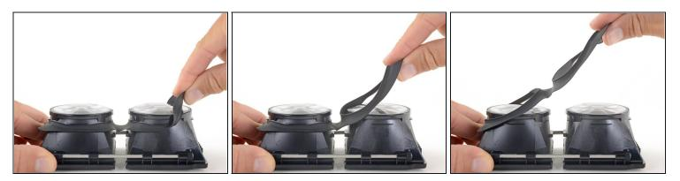
• Gently lift the eyepiece gasket off of the lens and OLED frames to remove it.
