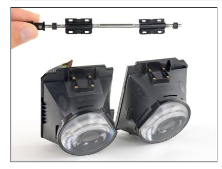
• Remove the focus rod and its brackets.
