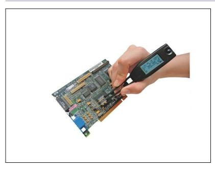
Now that an offset has been stored, Capacitance can be measured more accurately.
