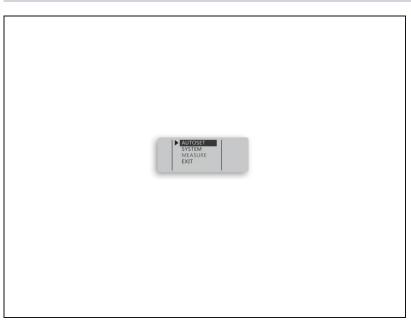
When you are finished measuring, make sure to reset the offset and custom settings by selecting the menu, then pressing AUTOSET.
