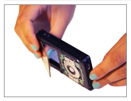
Grasping the sides of the cover, gently press on screen protector from the inside of the front cover to pop out the screen protector.
