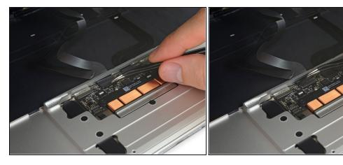
• Use tweezers to peel back the tape covering the trackpad cable ZIF connector.
