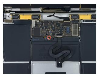
Remove the single 2.9 mm T5 Torx screw securing the battery connector to the logic board.
