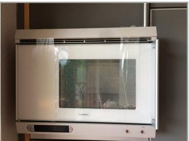
Pull the oven out of the cabinet by about 10-15cm (4" to 6" inches). Secure the door with some tape to the top of the oven.
