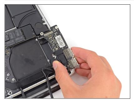
• Lift the I/O board straight up, out of the device.
