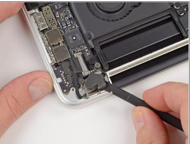
Use the flat end of a spudger to pry off the two rubber hinge covers, one from each end of the device.
