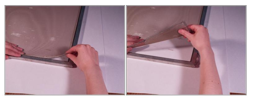
• Starting at an edge of the screen mesh, pull it upward to remove the mesh from the frame.
