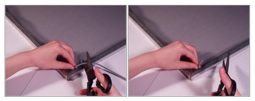
• After pushing spline into the frame channel on all sides, cut the end of the spline.
