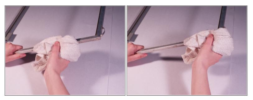
• Clean the frame using a warm, wet washcloth to remove dirt and debris.
