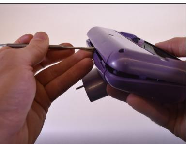
Separate the motorized brush face plate by using a flat prying tool.
