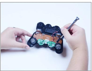
Remove the two 6.1 mm screws holding the internal analog stick board and the front of the controller together.
