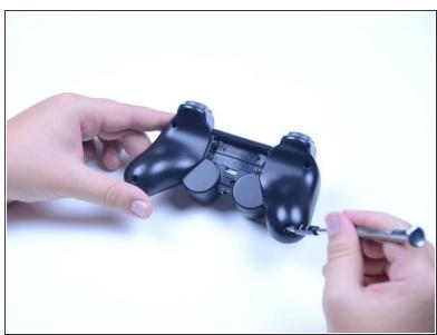
Remove the six 7.8 mm anchoring screws from the back casing of the controller using a Phillips #0 screwdriver.
