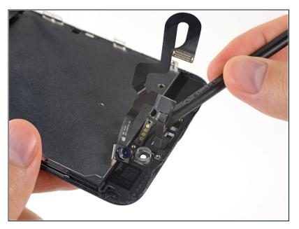
• Continue using your spudger to carefully separate the last of the flex cable from the back of the display.
