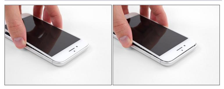
• Slide the display assembly slightly down (away from the top edge of the phone) to disengage the clips holding it to the rear case.
