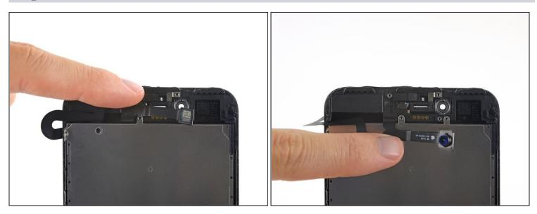
• Gently fold the camera and attached ribbon cable toward the bottom of the iPhone to allow access to the components underneath.
