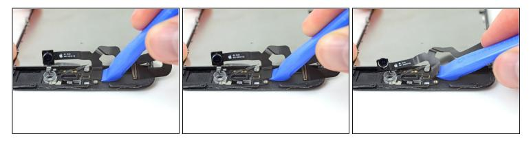
• Insert the sharp edge of an iFixit opening tool underneath the camera assembly's flex cable, on the opposite side from the front-facing camera.
