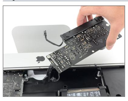
Remove the power supply from the iMac.
