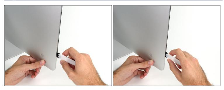
• Starting on the left of the display, near the power button, insert the iMac Opening Tool into the gap between the glass panel and the rear enclosure.
