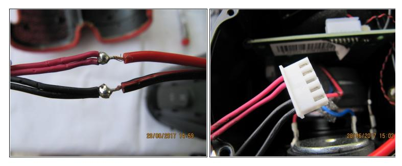
Solder the positive wires together, and solder the negative wires together. Use a 5.5 x 2.1 hollow DC connector for the power supply. Insulate the cable ends (Heat shrink wrap, electrical tape, etc.)
