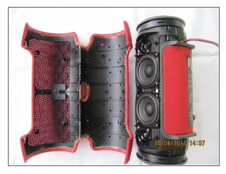
• Unscrew the screws and remove the shell.
