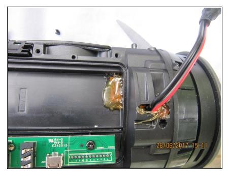
Remove the battery pack by unscrewing the 8 screws. Unplug the battery pack. Drill a hole. Seal holes with hot glue for air-tightness.
