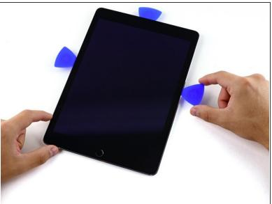
Opening picks are an industry favorite for maintaining a separation between screens and cases, or for breaking up long sections of adhesive. Feel free to explore your options.
