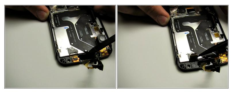
• Using a spudger, lift up the digitizer cable that is attached to the glass.
