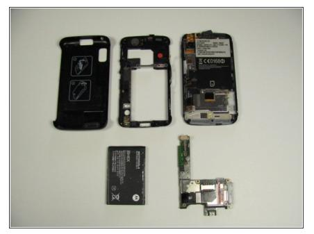
After disconnecting the motherboard, there should be five distinct and separate parts of the phone: back cover, back case, front case, battery, and motherboard.
