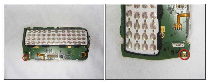
• The microphone is located on the bottom corner of the motherboard.
