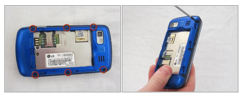
Unscrew the six 2.4mm Phillips #00 screws (three on the left and three on the right of the phone) to remove the inner back case.
