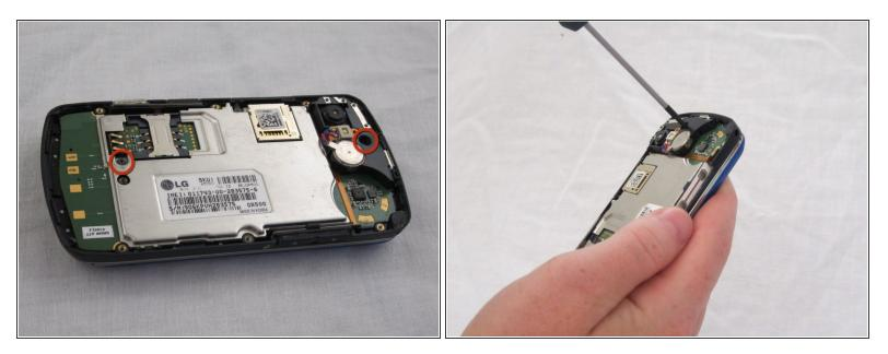
Carefully remove the two 3mm Phillips #00 screws (one on the top and one on the bottom) that are attaching the motherboard to the phone.
