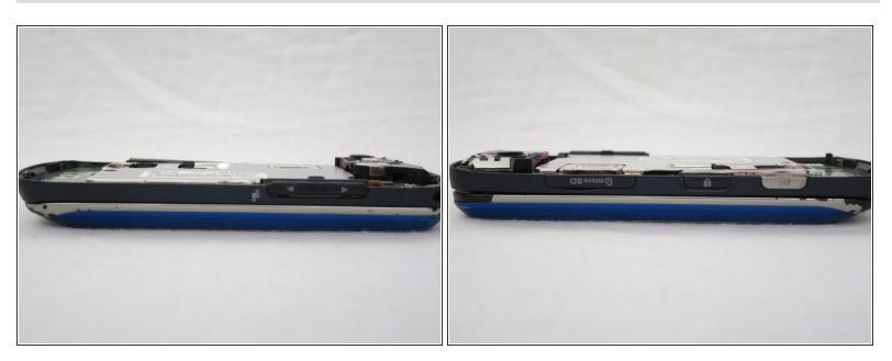
• Remove the camera, lock, and volume buttons from the side of the phone.
