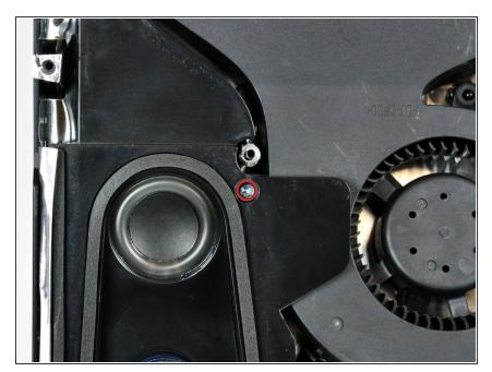
Remove the single T10 Torx screw securing the left speaker to the rear case.
