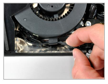
De-route the left speaker cable from the channel in the CPU fan.
