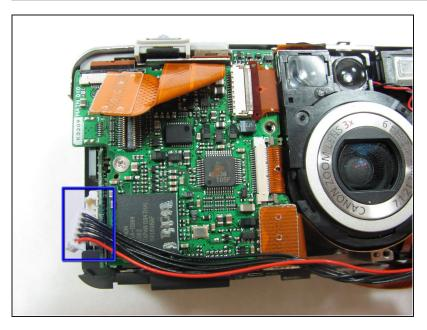
Disconnect the black and red cable on the left side of the lens.
