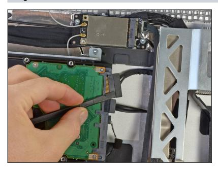
Using the flat end of a spudger, remove the SATA power cable from its socket on the hard drive.
