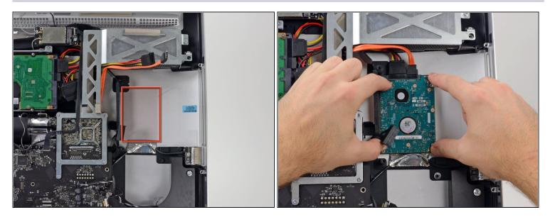
• After removing the backing from the adhesive pads, press the secondary hard drive firmly against the aluminum frame of the iMac.
