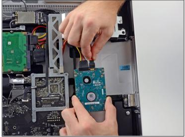
Connect the SATA power and data cables to the secondary hard drive.
