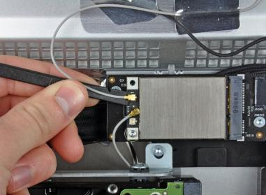
• Use the flat end of a spudger to pry both AirPort antenna cable connectors up off the AirPort card.
