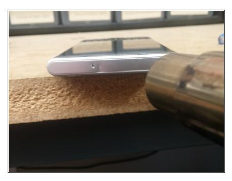
Apply heat to the top of the phone to remove the microphone plastic cover. There is a fair amount of adhesive holding this cover down.
