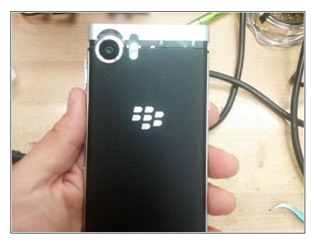
The plastic top of the phone will slide off after removing the two screws.
