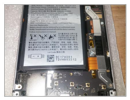
Removing the loud speaker cover will allow you to remove the other two Phillips screws for the metal bracket that covers up a couple flex connectors.
