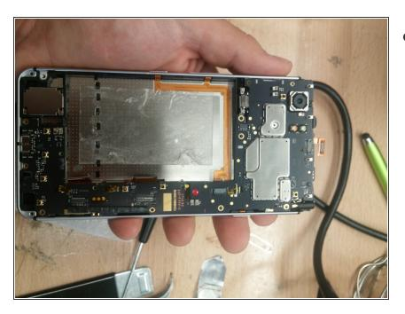
With all screws and brackets removed and all flex cables disconnected you can now remove the motherboard. I recommend starting at the top (Rear facing camera side) and removing the board top down because the charging port sits in the frame of the phone and will come out more easily last.
