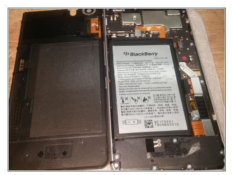
Once the back cover is off remove the 7 Phillips Screws at the bottom of the phone that are covering the loudspeaker and the part of the motheboard where the USB type-C charging port is located.
