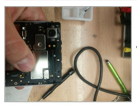
There are three Phillips screws holding down a black plastic bracket that was previously partially covered by the silver bracket removed earlier. Two of the screws are visible without removing the silver top bracket but the third middle screws requires the top bracket be removed first.
