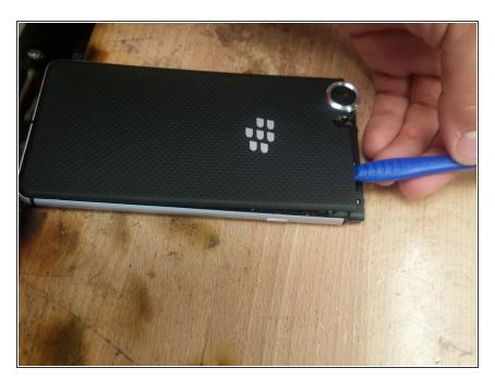
With the top plastic cover off it is pretty easy to use your preferred plastic pry tool and remove the battery cover.
