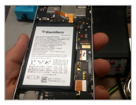
Disconnect the two Phillips screws connecting the battery flex connector to the motherboard. Now you can remove the battery. There is ALOT of adhesive holding the battery in place. I recommend applying heat and using a plastic tool to slowly work the battery out. The volume and power flex runs under the battery. Be cautious near the top left.
