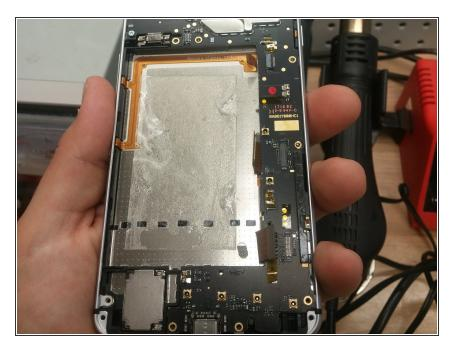
With the battery out disconnect the three flex cables and remove the remaining two Phillips screws from this area of the motherboard.
