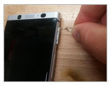
Use a sim card removal tool to remove the sim card.
