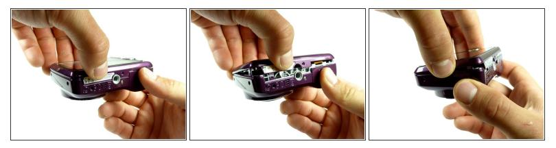
• Once all the screws are out, remove the back panel.
