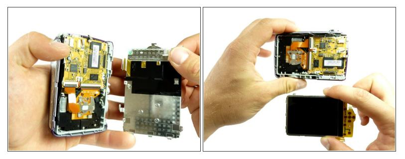
• The LCD screen is now completely removed from the rest of the camera.
