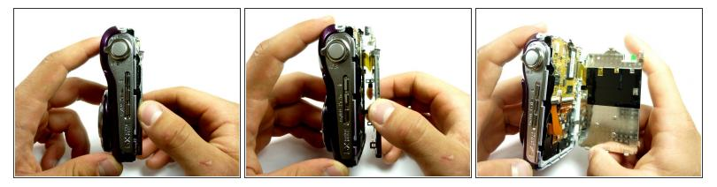
• Carefully pry the top portion of the screen from the camera.
