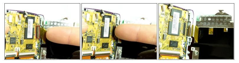
• To remove the screen completely, push down on the rectangular tab indicated in the picture.
