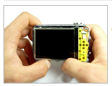
In the top right hand corner of the inside of the camera, there is a Philips #00 4 mm screw that needs to be removed.
