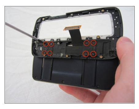
After removing the motherboard and keyboard, unscrew eight 1.6mm
