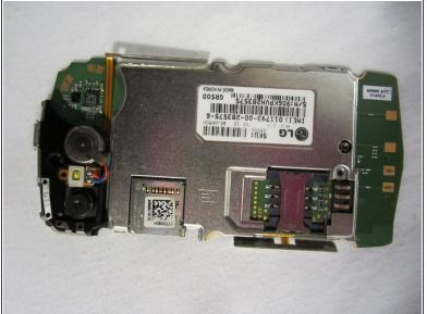
Once the cable is removed, you have successfully disassembled the motherboard of your phone.
