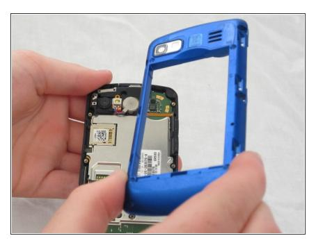
Once all six screws are removed, use the plastic opening tool to carefully pry apart the inner back case. Push the plastic tool underneath the case. Carefully push upward, with the tool, while moving it around the case.
