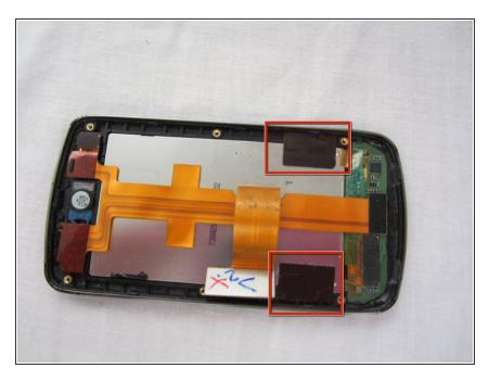
Remove the black electrical tape holding the LCD to the screen.
