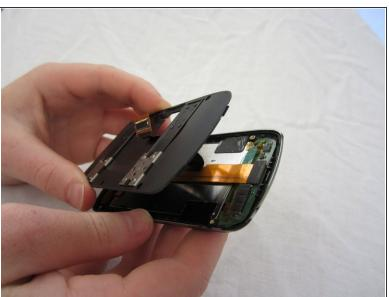
Using the plastic opening tool, carefully open and remove the case. Slide the tool along the edge and pry upwards to open.
