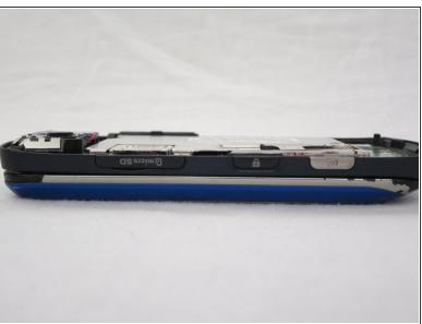
Remove the camera, lock, and volume buttons from the side of the phone.
