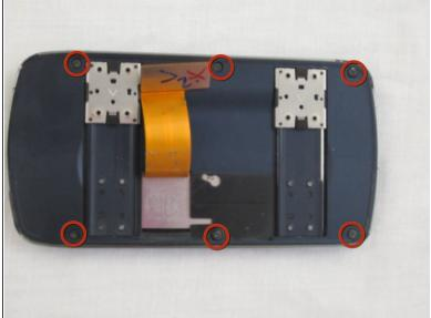
Remove six 2.25mm Phillips #00 screws along the outside of the case.
