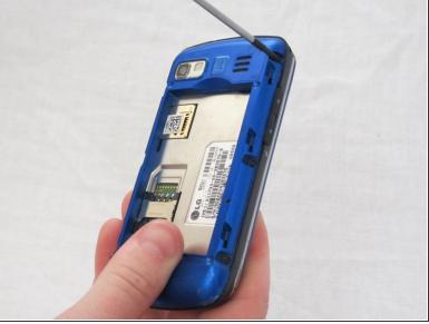
Unscrew the six 2.4mm Phillips #00 screws (three on the left and three on the right of the phone) to remove the inner back case.
