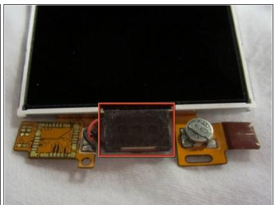
The speaker is attached to the top of the LCD.
