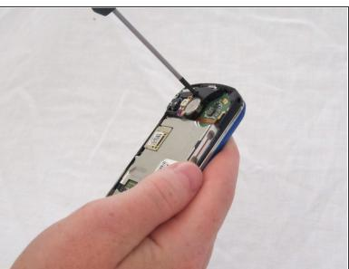
Carefully remove the two 3mm Phillips #00 screws (one on the top and one on the bottom) that are attaching the motherboard to the phone.
