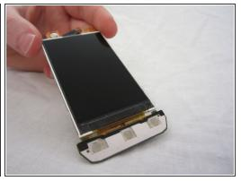
Unhook the LCD from tabs on the bottom using the plastic opening tool.
