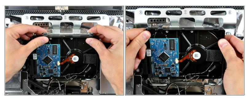
• Rotate the top of the drive toward yourself, then lift the hard drive straight up off its lower pins.
