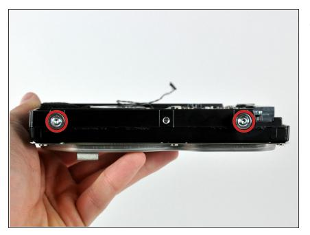
Remove the two T8 Torx screws and their attached rubber grommets from the hard drive.
