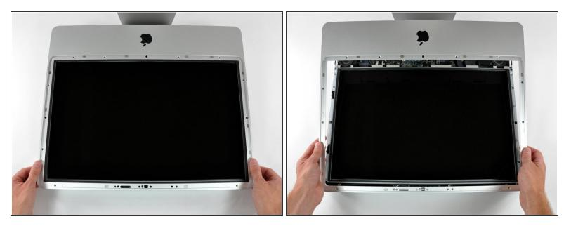
$\bigwedge$  The front bezel is still attached to the iMac by the microphone cable.
