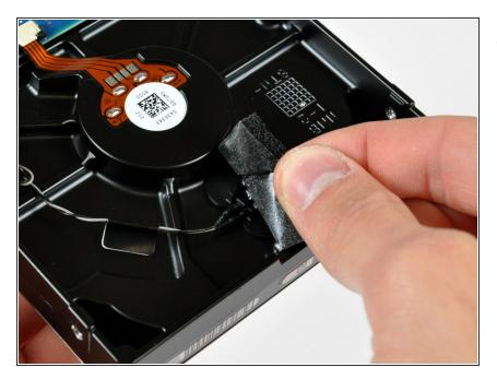
Peel off the piece of foam tape covering the hard drive thermal sensor.
