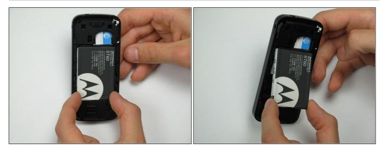
• Pinch the sides of the bottom of the battery and pull upward.
