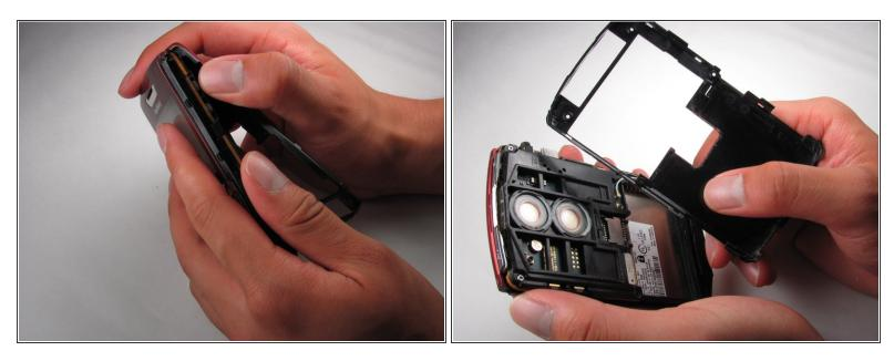
• Remove the back casing using the Plastic Opening Tool
