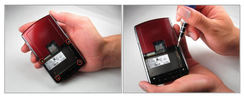
• Once the battery is removed, remove the four 9.2 mm screws with the T4 Torx Screwdriver.
