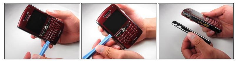
• Remove side panels with the Plastic Opening Tool by sliding it along the edge of the panel until you can pry it off with the tool.
