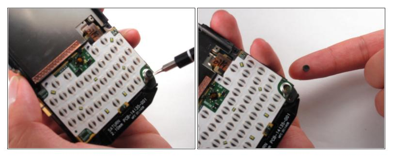
Once the microphone is revealed, use the flathead screwdriver, or the tip of a knife, to carefully pry the microphone out of the hole.
