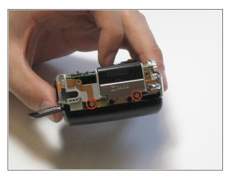
Remove the two 3.0mm screws on the right side of the camera.
