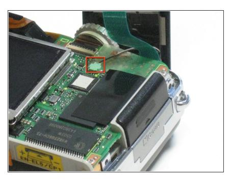
Disconnect the cable by pulling the head upward along the green circuit board. If you only are changing the LCD, skip this step.
